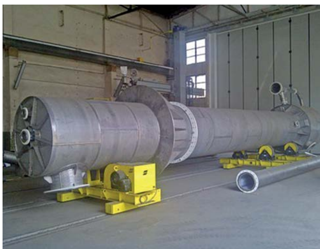
Reactor; \varnothing 1.5 \text{ m} ; H = 20 \text{ m} ; Weight \approx 7 \text{ t} Titanium grade 2 and grade 7
