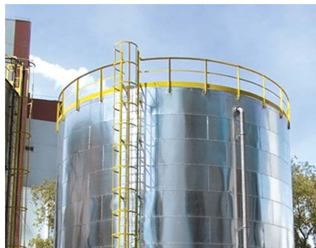
Chemical Waste Reactor; Ø 10 m; H = 11.5 m; Weight ≈ 30 t
