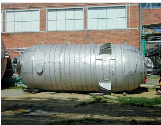
Reactor; \varnothing 2.6 \text{ m} ; L = 8 \text{ m}
