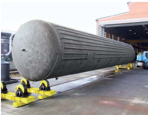
Storage tank; V = 200 \text{ m}^3 ; \varnothing 3.4 \text{ m} ; L = 23 \text{ m} ; Weight \approx 43 \text{ t}
