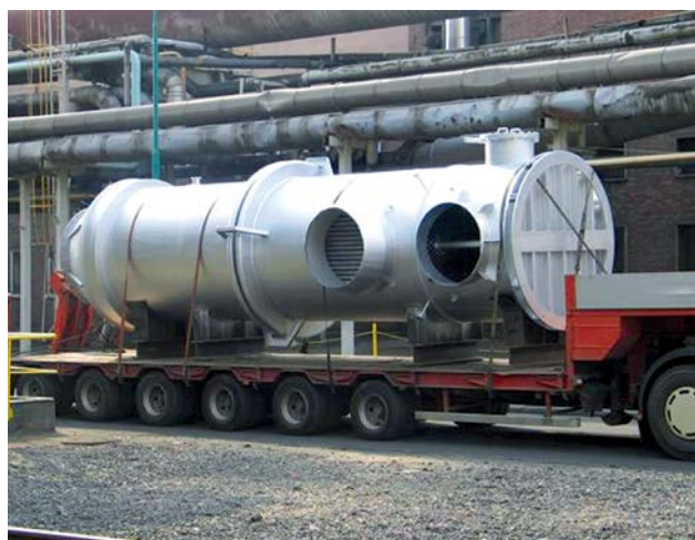
Heat exchanger; \varnothing 2.0 \text{ m} ; L = 9 \text{ m} ; Weight \approx 26 \text{ t}
