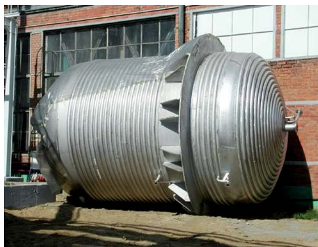
Reactor; \varnothing 3.5 \text{ m} ; L = 7 \text{ m}
